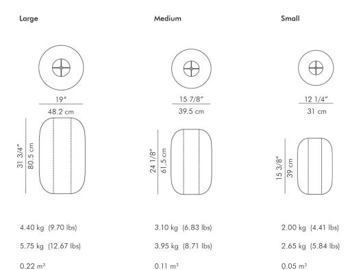
Surface mounted pre-wired lamp E26 / E27 120V 60Hz / 230V 50Hz 1 x 100 watts | 1 x 100 watts | 1 x 75 watts
