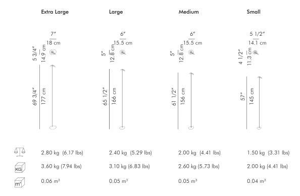
Portable pre-wired lamp 100-240 VAC 50/60 Hz LED 0.48 watts
